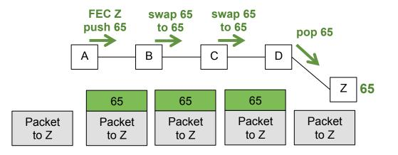
A packet injected anywhere with top label 65 will reach Z via shortest-path
