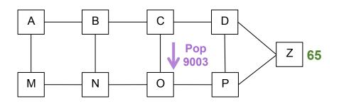
A packet injected at node C with label 9003 is forced through datalink CO
