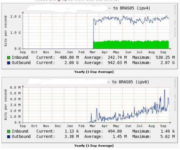
To see IPv6 traffic in MRTG, we've forwarded traffic separately via two interfaces. On both interfaces we have Dual-Stack but with different OSPF cost for IPv4&IPv6.
